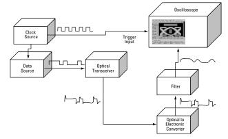
Figure 1: Test setup with external clock source available.
