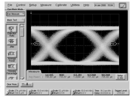
Figure 12: Average power measurement with Agilent 86100A.
