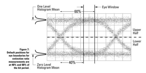
Changes in extinction ratio measurements for the Agilent 86100A Infiniium DCA in comparison to the Agilent 83480A
