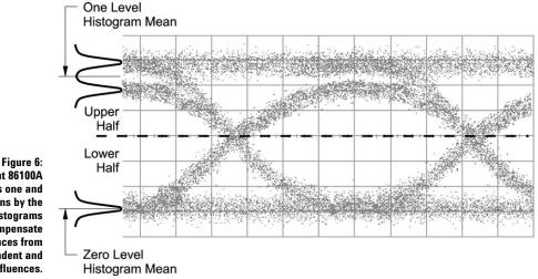
The Agilent 86100A determines one and zero level means by the use of histograms which compensate for variances from pattern dependent and noise influences.
