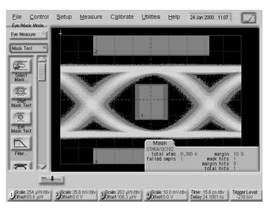
Figure 4: The Agilent 86100A allows the user to define mask margin percentage. Note that acutual failed samples are tabulated separately from those samples which passed the mask test but fell within the mask margin area.
