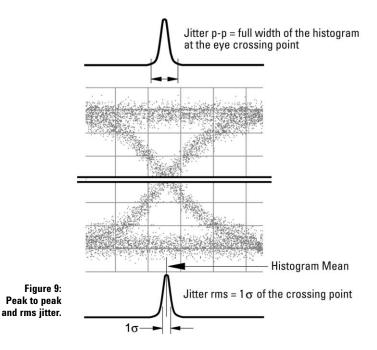
The 86100A creates histograms to find the crossing point of the eye diagram and then takes a very narrow sample in the horizontal axis at the vertical level of the crossing point. The time difference between the end samples of this sampling window constitute the peak to peak jitter measurement. The rms jitter is found by constructing a histogram of the samples between the end samples and determining the mean and standard deviation of the distribution of the samples.
