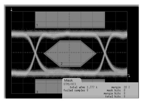
**Extinction ratio** Extinction ratio is defined as the ratio of the mean one level divided by the mean zero level of an eye diagram. Extinction ratio can be expressed in one of three ways:
