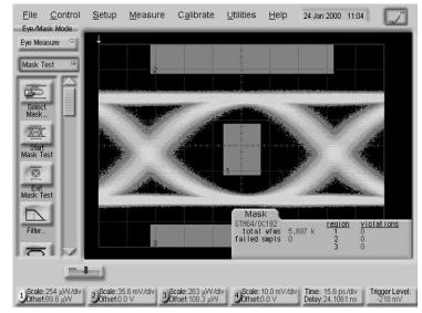
Figure 3: Mask test shown on Agilent 86100A.
