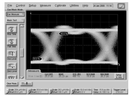
Figure 11: Agilent 86100A rise time measurement.
